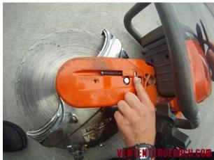
NOTICE TENSION THE DRIVE BELT BY SCREWING IN THE TENSIONING SCREW FAR ENOUGH SO THAT THE INDICATING SQUARE NUT COMES OPPOSITE THE ARROW.
