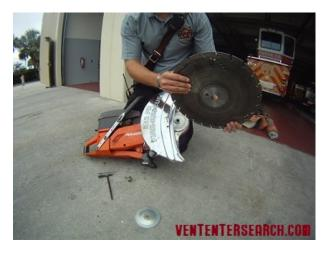
9. REMOVE THE BOLT AND DISC PLATE. FLIP THE CUTTING BLADE 180 DEGREES.
