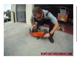
1. LOOSEN THE TENSIONING SCREW SO THAT THE BELT TENSION RELEASES.
