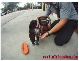
4. INSERT CUTTER ARM INTO THE OUTBOARD SLOT OF THE SAW.
