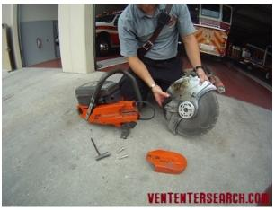
3. REMOVE THE BELT GUARD AND CUTTER ARM.
