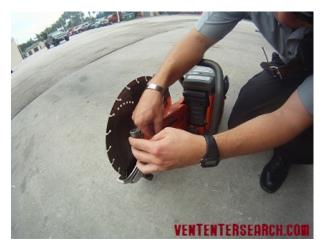
7. TENSION THE DRIVE BELT WHILE ROTATING THE BLADE BY HAND, THEN GO BACK AND TIGHTEN THE NUTS.
