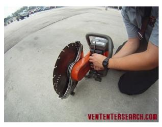
6. TIGHTEN THE NUTS HALF WAY.
