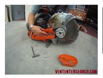
NOTICE THE MANUFACTURE HAS MOLDED A SLOT FOR THE SAW TO BE USED AS AN OUTBOARD.
