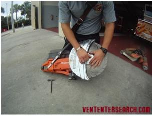
10. REPLACE THE CUTTING BLADE, DISC PLATE AND BOLT, TIGHTEN ASSEMBLY.
