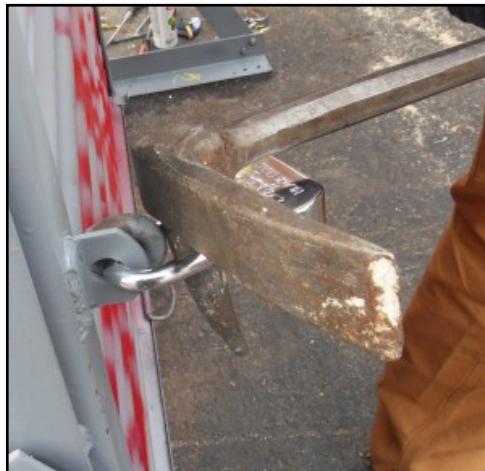
Picture 6. Using a haligan point to defeat a pad-lock. (Photo courtesy of Traditions Training)
